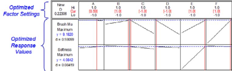
Experimenters used the Minitab Response Optimizer to determine the optimal configurations for eliminating brush marks and maintaining carpet plushness at the same time.
